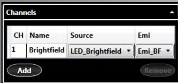
Fig. 5: Channels Choose your required light source, dichro (Cellavista® only) and emission filter.
