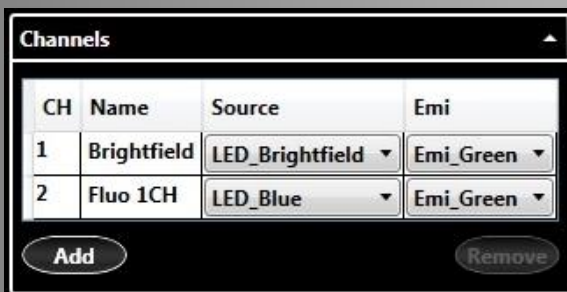
Fig. 5: Channels Choose your required light source, dichro (CELLAVISTA® only) and emission filter.
